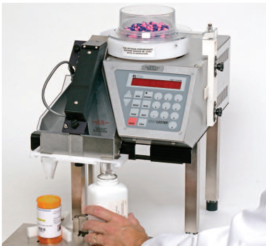
This adjustable-speed counter-filler handles as many as 1,920 tablets or capsules per minute and is suitable for packaging and batch verification applications.
